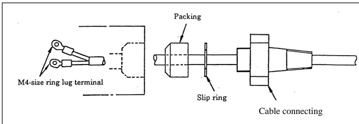
**Figure 4.8 Cable connections**
