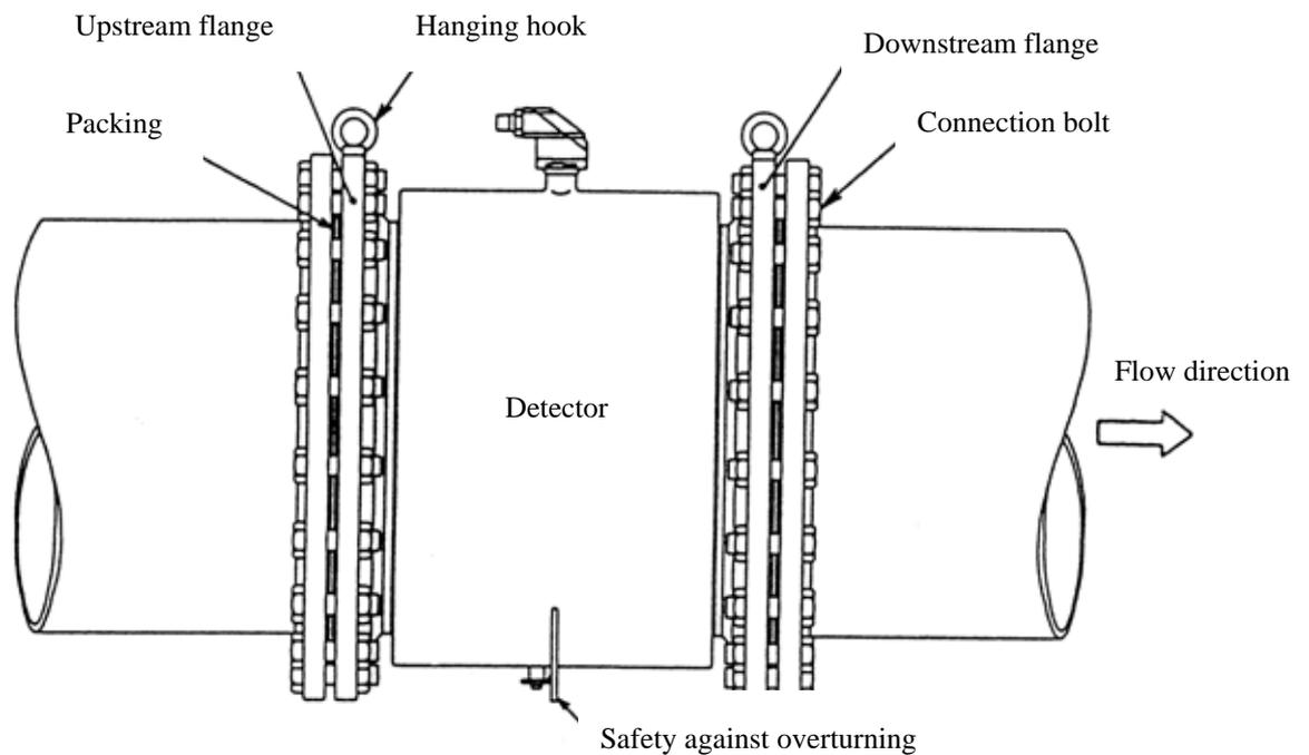
**Figure 4.1 The LF150 detector piping connections**
