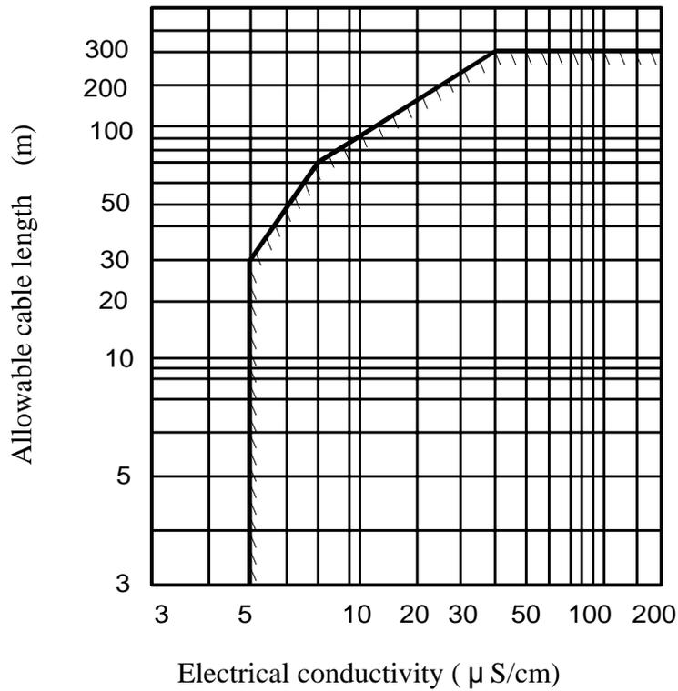
**Figure 8.1 Electrical Conductivity vs. Cable Length**
