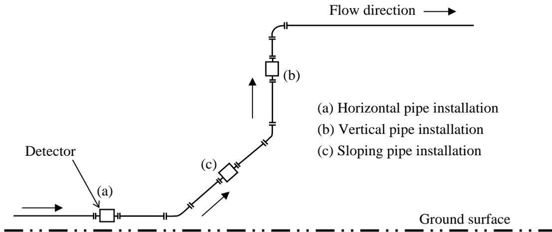
**Figure 4.2 Detector Piping Orientation**
