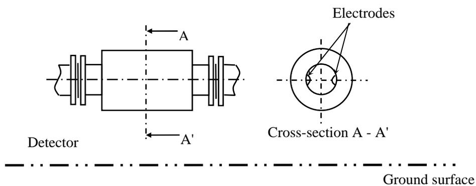
**Figure 4.3 Installation position of the detector**
