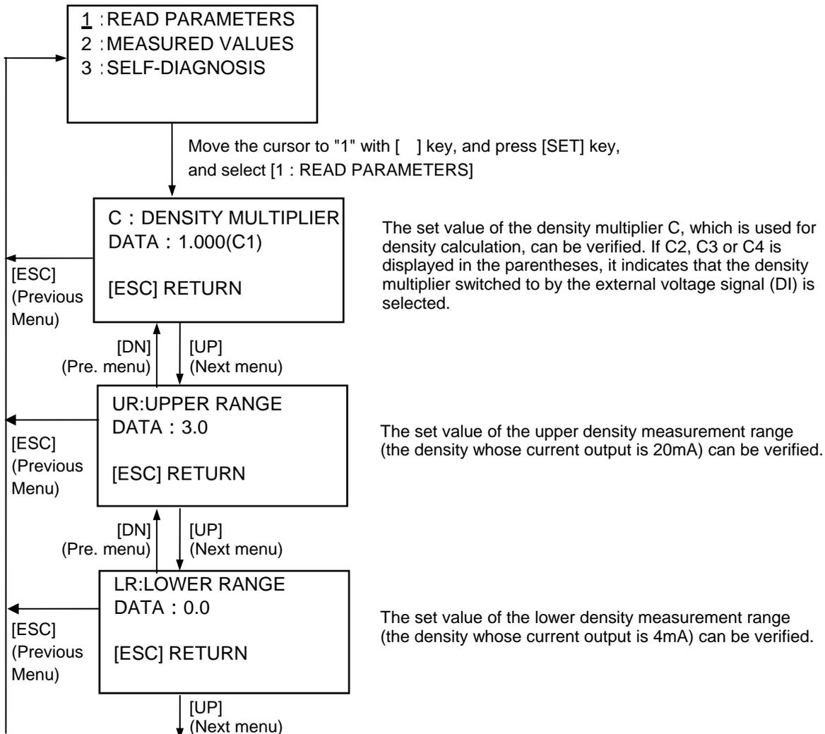
The set value of the density multiplier C, which is used for density calculation, can be verified. If C2, C3 or C4 is displayed in the parentheses, it indicates that the density multiplier switched to by the external voltage signal (DI) is selected.
