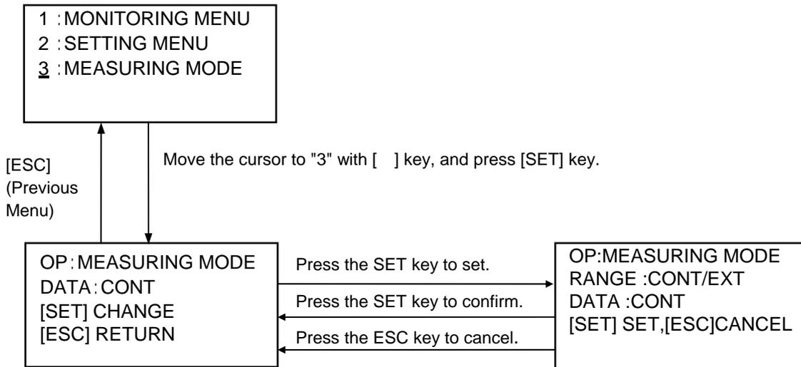
Each time the ° [UP] or [DN] key is pressed, CONT/EXT are mutually alternated thus making it possible to select an operation mode. Select "CONT" for normal continuous operations; select "EXT" for external synchronized operations. For details on the external synchronized operation, refer to Section 6.7.
