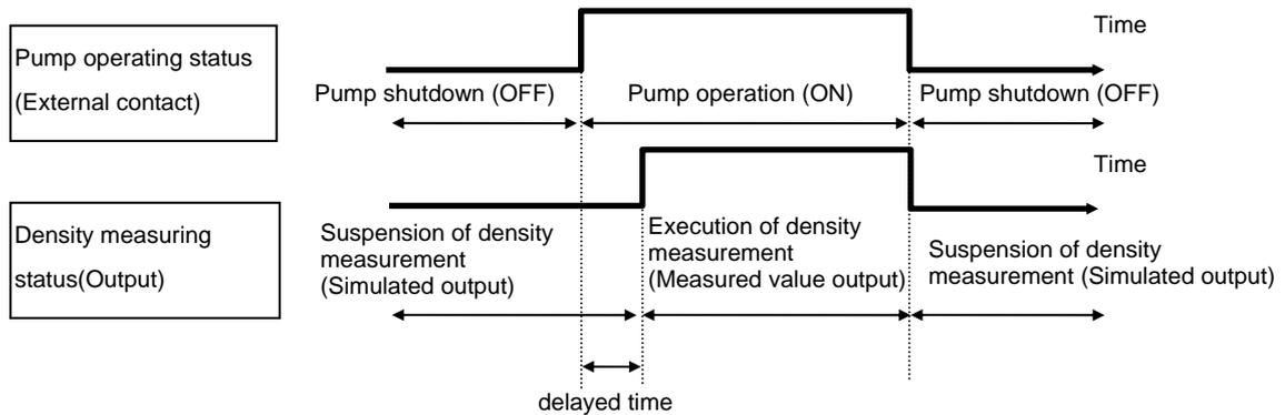
**Figure 6.7.1 External synchronized Operation**
