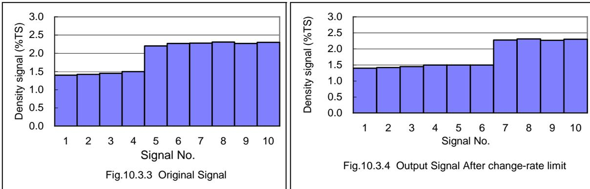
Figure 10.3.3 shows the original signal before the change-rate limit is processed. The numeric values along the horizontal axis refer to the signal numbers. No.1 to No.4 are varying within a small width; however, signal No.5 is varying in excess of 0.5%TS with No.6 to No.10 remaining in a state not very different from No.5.
