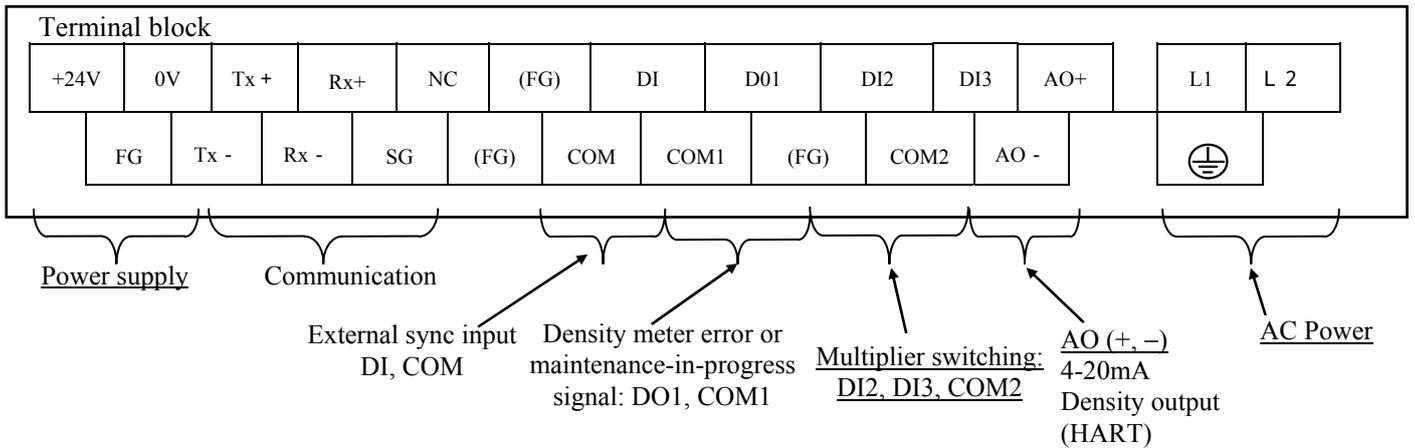
**Figure 4.5.2 Terminals inside the converter**
