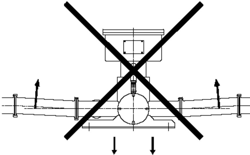
Since the stagnant liquid may stay in the piping section, do not install the density meter in a position where the cover of the applicator sections (transmitter side and receptor side: see Figure 3.1.1) is level (applicator sections are in upper and lower positions).
