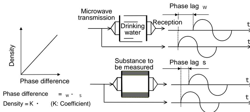
Figure 1.1 Principle of phase angle difference
