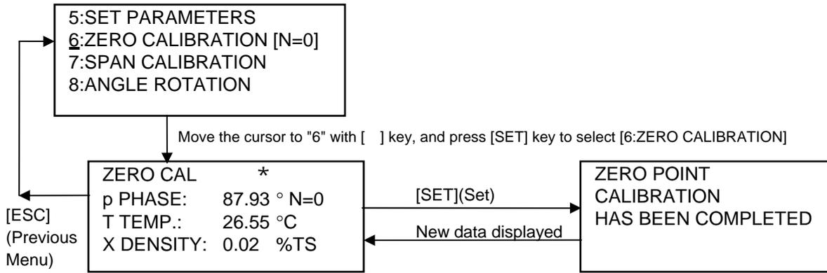
Press the [SET] key for zero calibration. In zero calibration, the phase and the fluid temperature of zero point will be replaced with the present measured values. And also, angle rotation "N" will be set to zero.
