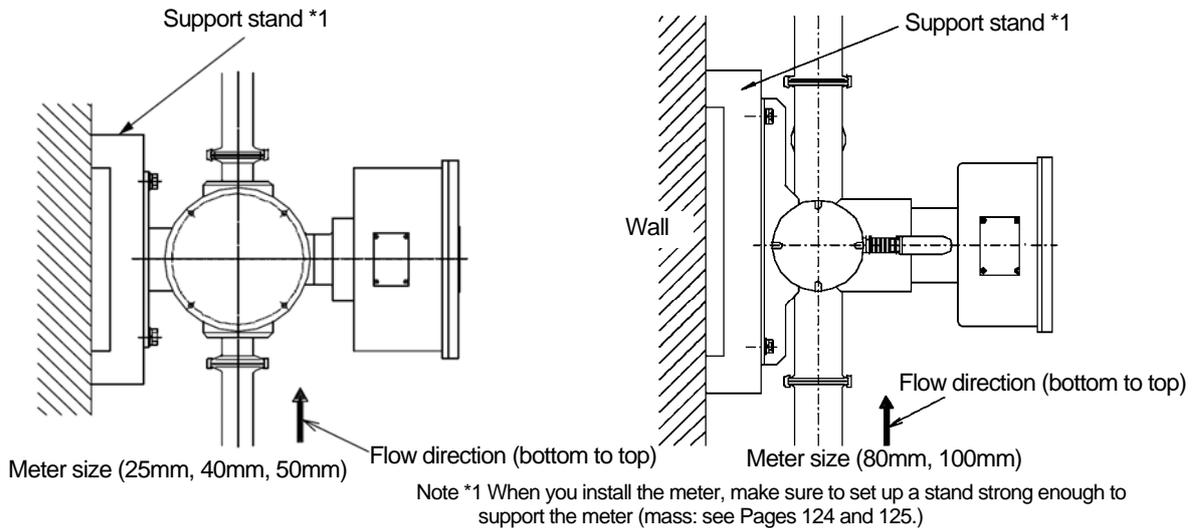
**Figure 4.3.2 Example of Detector Pipe Installation (Vertical Piping)**
