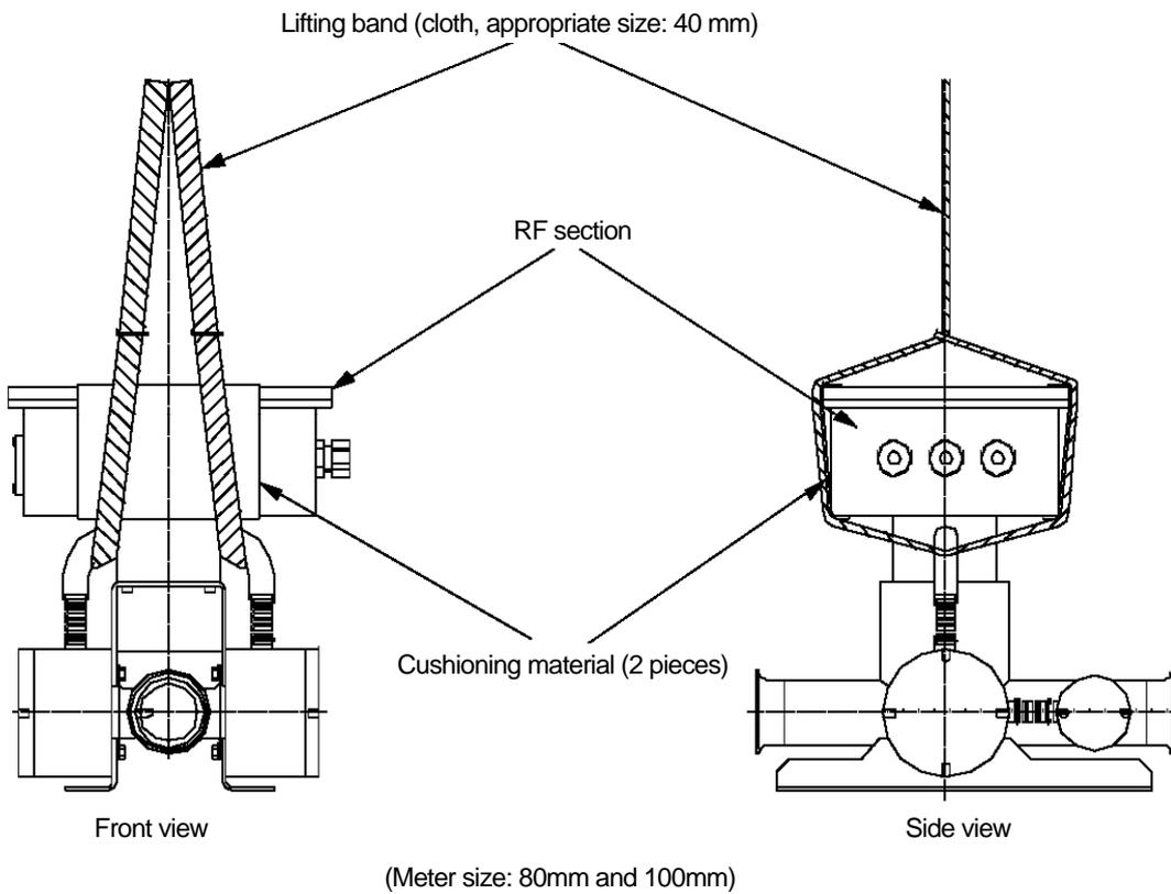
**Figure 4.1.2 Procedure to Lift the Density Meter in Horizontal Position**
