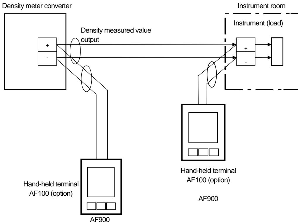
**Figure 4.5.4 External Connection Diagram**
