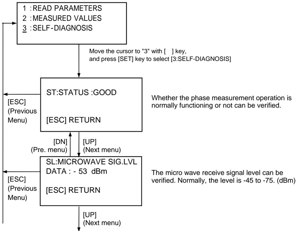
Whether the phase measurement operation is normally functioning or not can be verified.
