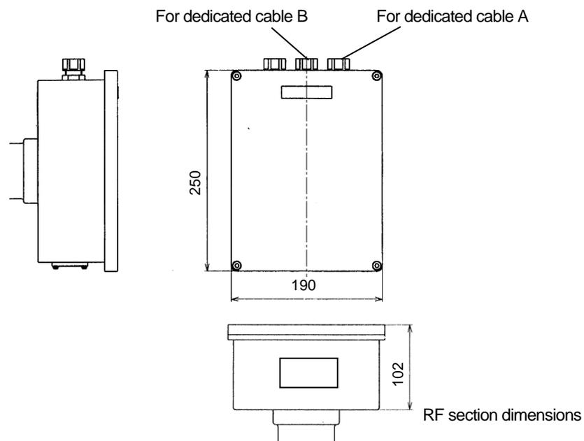
Attached Figure2. Converter dimensions
