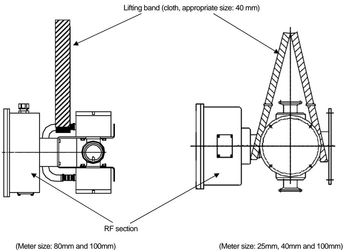
**Figure 4.1.1 Procedure to Lift the Density Meter in Vertical Position**
