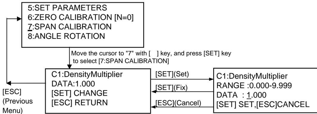
The density multiplier C1 should be set to the suitable value so that the measured density value is corresponding to the manual analysis value. For details, refer to Section 6.5.
