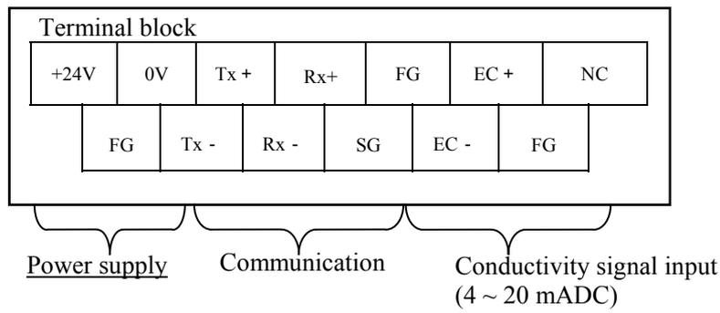
**Figure 4.5.3 Terminals arrangement inside the RF section**
