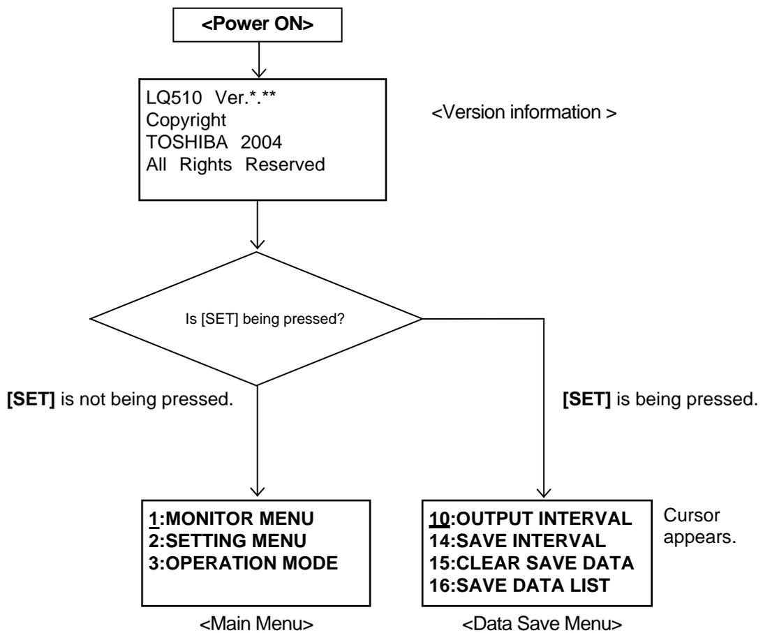
Figure 10.8.1. Maintenance Menu Starting Method
