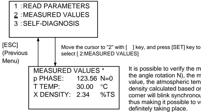
It is possible to verify the measured phase value (and the angle rotation N), the measured fluid temperature value, the atmospheric temperature, as well as the density calculated based on them. [\*] in the upper right corner will blink synchronously with the data updating thus making it possible to verify that the data updating is definitely taking place.
