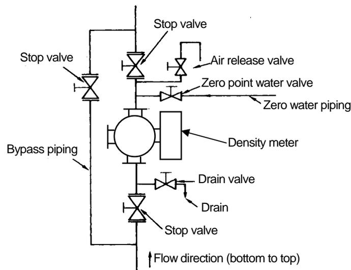
**Figure 4.3.3 Example of Detector Installation (Vertical Piping)**
