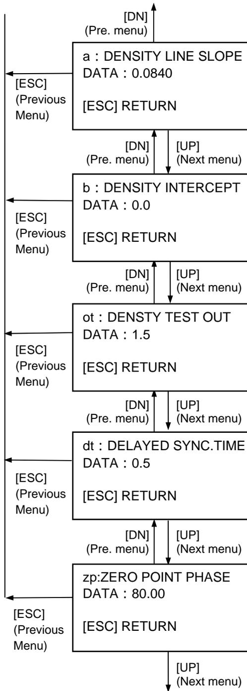
The set value of "density line slope" of the arithmetic expression for calculating the density from the phase measurement data, etc. can be verified.
