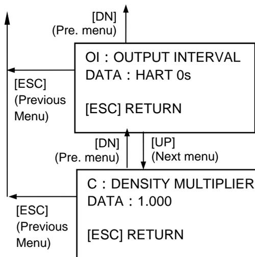
Which type of communication method is selected, HART communication<sup>1</sup> or RS232C communication<sup>2</sup>, can be checked and also the output interval can be checked.
