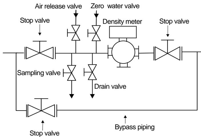
**Figure 4.3.5 Example of Detector Installation (Horizontal Piping)**
